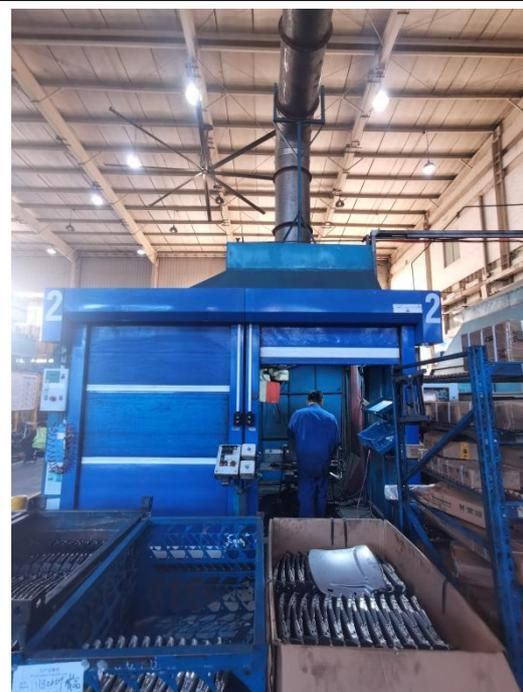
焊接工序柜式集气罩
